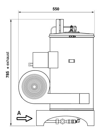
WHU water heater, producing hot water or steam, is ideal in demanding cleaning tasks. High water temperature greatly enhances impact effect and water jet scouring capacity.
